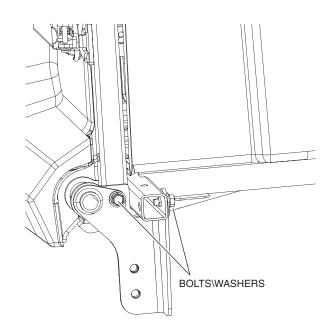
Align the rear bumper to hinge brackets and attach with four 8 mm bolts. Two on driver side and two on passenger side. Tighten bolts to the values found in the torque chart.
