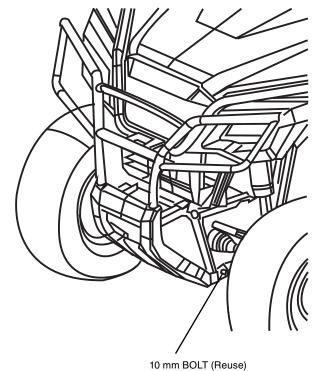
7. Tighten all hardware to values specified in the Torque Chart.
