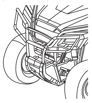
5. Loosely install the bumper using the supplied P-bracket, 10 mm bolt, nut, and washers. Use a washer on each side of the P-Bracket. Loosely install the two upper 8 mm bolts and nuts.
