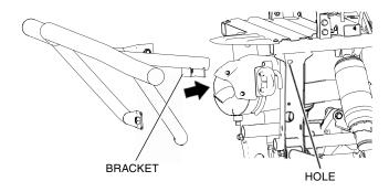
2. Lossely install the 10 x 20 mm bolt and washer from the other side as shown.
