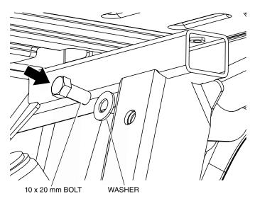
3. Loosely install the 10 x 20 mm bolt and washer on the top left side as shown.
