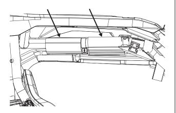
8. Use a aelf-tapping phillips head screw and the original bolt to secure the bracket on the Fabric Upper Door to the original door and tighten.
