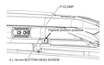
11. Wrap the upper strap on the Fabric Upper Door around the vertical OPS at the highest position possible then tighten.
