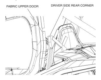
20. Attach the Fabric Upper Door, the driver side rear corner, and the Rear Panel (if installed) using the hook and loop sections (as shown).
