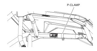
5. Install two C-clamps on the vertical OPS tube (as shown).
