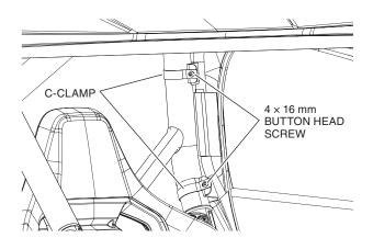
13. Install the original net on the door using the original hardware and a  $4 \times 20$  mm button head screw, spring lock washer and fender washer (as shown).
