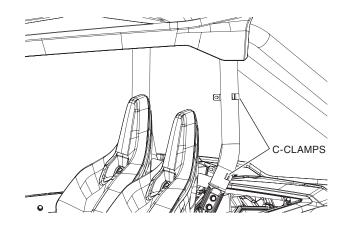
6. Place the Fabric Upper Door on the original door making sure the top section is under the original roof. Make sure the holes are lined up.
