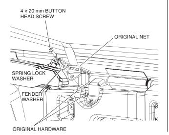
14. Install the original net on the door using the original hardware (as shown).
