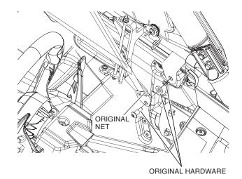
15. Wrap the front strap on the Fabric Upper Door around the front OPS tube then tighten.
