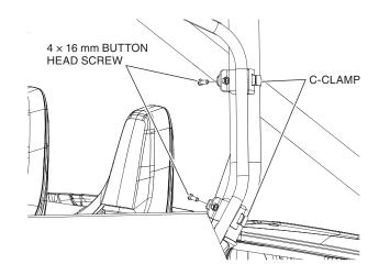
10. Install the Fabric Upper Door on the P-clamp at the highest position possible then tighten.
